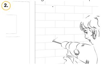
Remove the bracket and drill a hole at 10mm diameter and 50mm deep.
