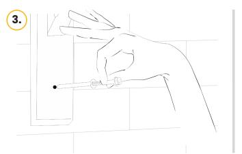
Then, reposition the bracket and knock in the plug and screw into place. Be sure to tighten both screws.
