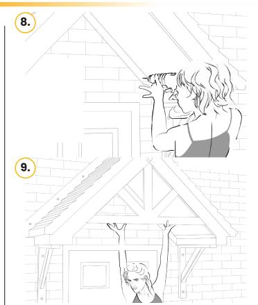
Insert the truss into the front of the canopy and fix it in place. If required, fit the ridge tiles at the peak of the apex.
